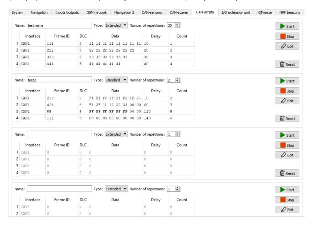
In the future, these scripts can be run using the SMS command or the Wialon IPS and Wialon Combine. CAN scripts are also used when setting up tracker scripts (see the "Scripts" section).
