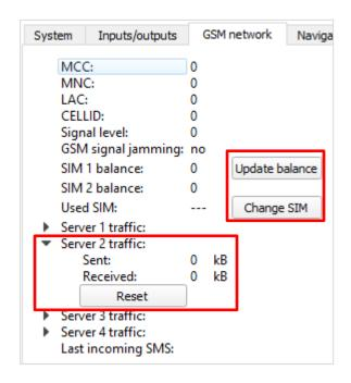
If you press the "Update balance" button, then the device updates the balance of active SIM according to the settings in the "Server connection" part.
