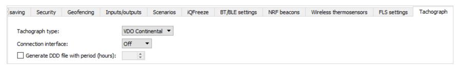
Here you need to specify the tachograph model, select the interface through which it is connected and set the period for generating the DDD file.
