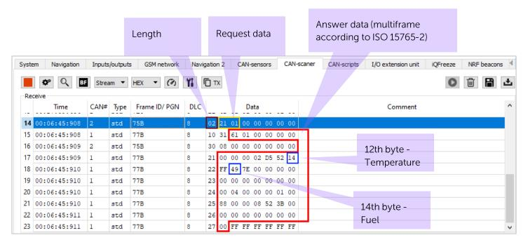
And in the CAN-sensors tab, the converted (according to the signal settings) sensor values will be displayed
