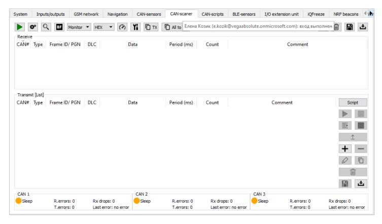
If the scanner is connected, you can press the start button "and then all information from the CAN-bus will be displayed in the "Receive" field, and instead of the start button the stop button "will appear. Consider the upper part of the window where the settings for displaying information from the CAN-bus are located and the information is displayed.
