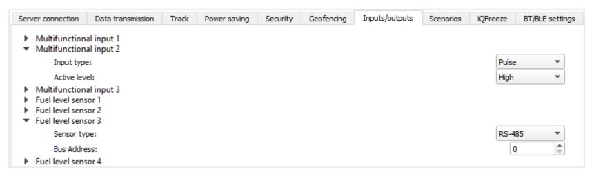
Fuel level sensor – the ability to connect up to 4 fuel level sensors via the RS-232, RS-485 or UART interface, specifying the address on the bus and selecting the appropriate "Sensor Type".
