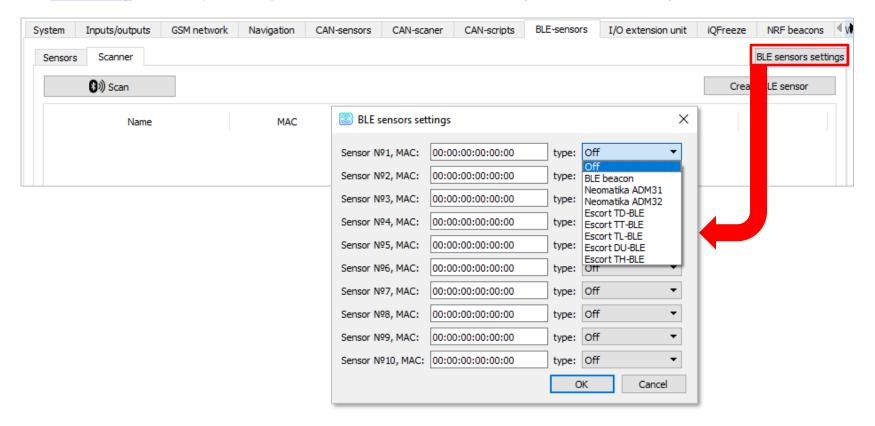
Supported BLE-sensors types are listed in the drop-down list.
