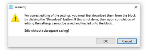
It also appears if the device was not connected at all. Therefore, before configuring CAN sensors, you need to load the settings from the device by clicking the "Download" button in the left part of the window.
