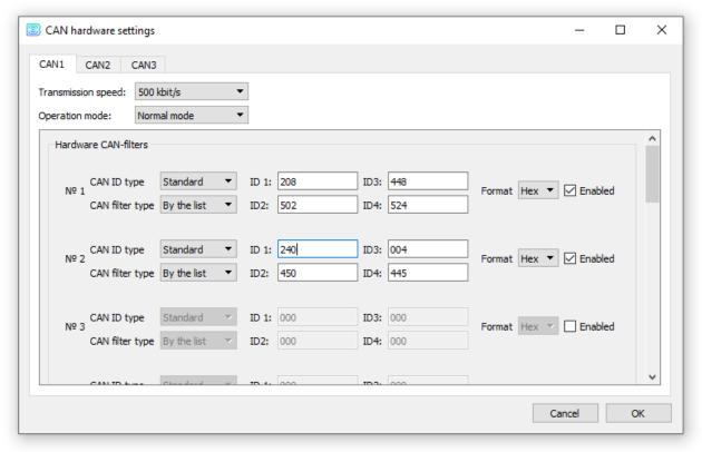
Transmission speed – it is important to indicate the correct speed for the CAN bus.
